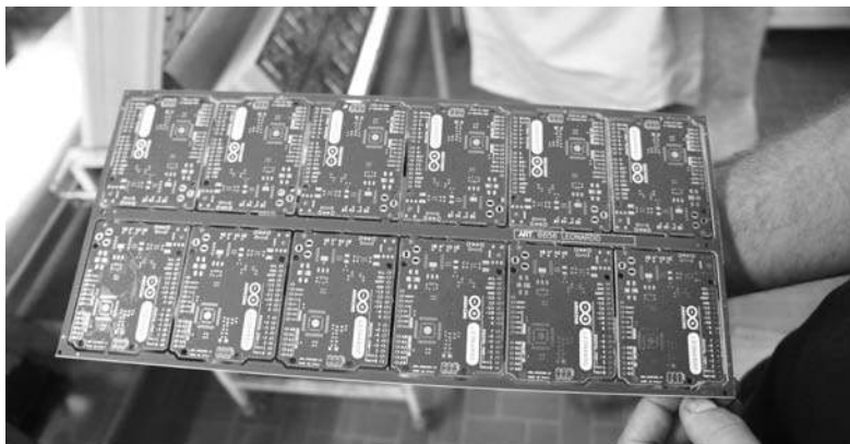
Smaller 2×6 panels make SMT processing more efficient.
