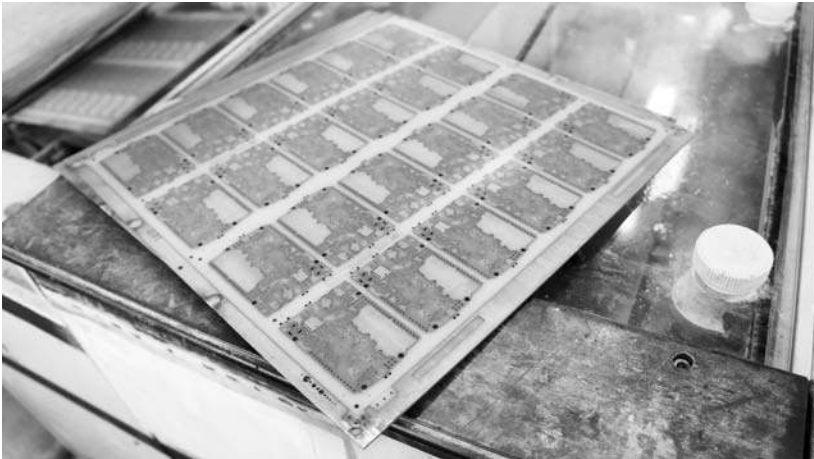
A panel etched of unwanted copper
