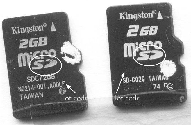
An irregular microSD card (left) and a normal card (right). The arrows show suspicious differences.
