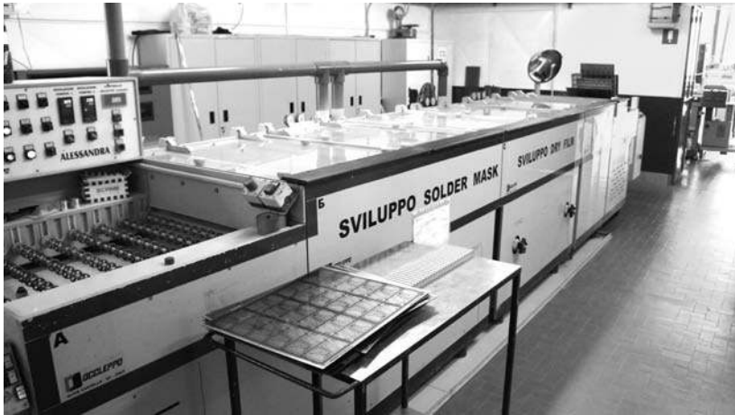
The machine that develops the photoresist
