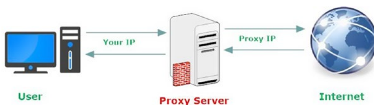
Figure 2-19. How a proxy server works (source: www.GarknessGate.com )
